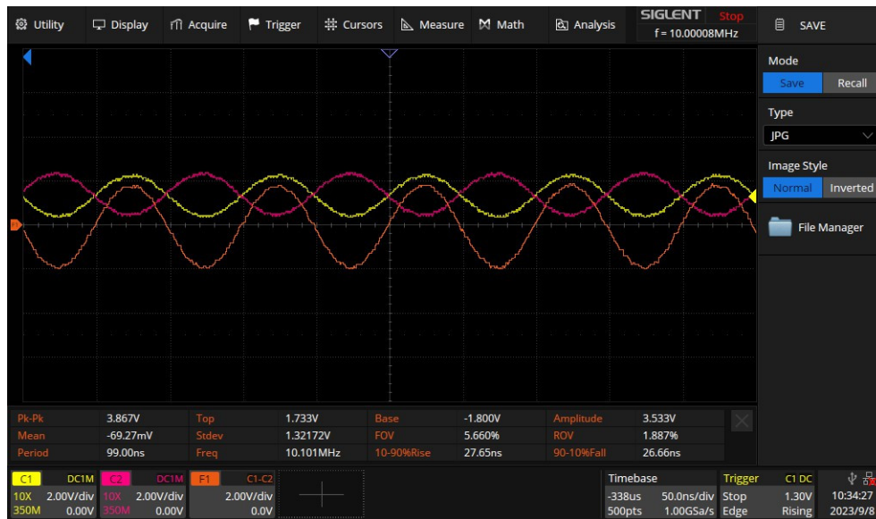
Figure 6: Produced waveform, measured at AFE0 output resistor R36A, R39A.
